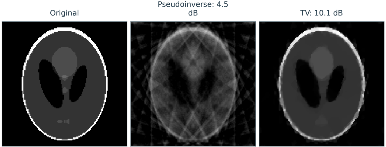
Figure 9.10. TV-regularized reconstruction and the pseudoinverse for the same partial Fourier measurements.
