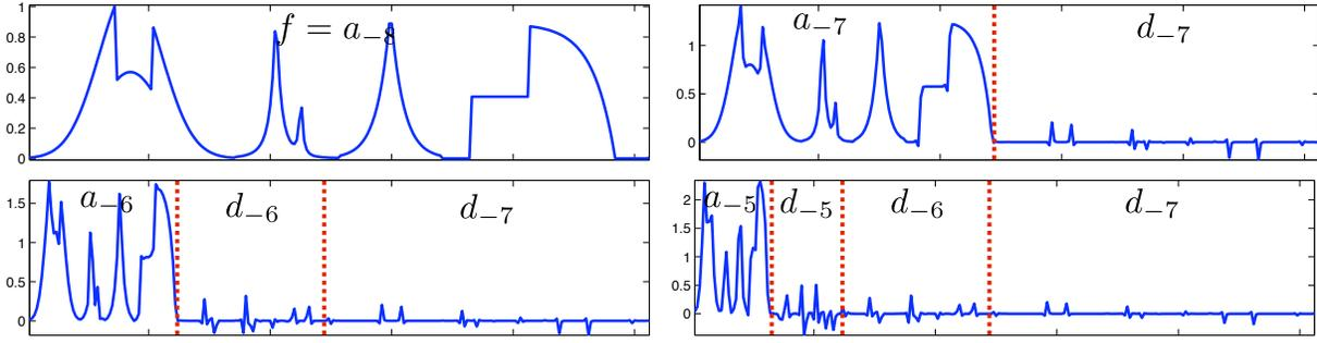
Figure 3.12: Wavelet decomposition algorithm.
