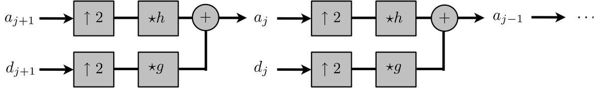
Figure 3.14: Backward filterbank recombination algorithm.
