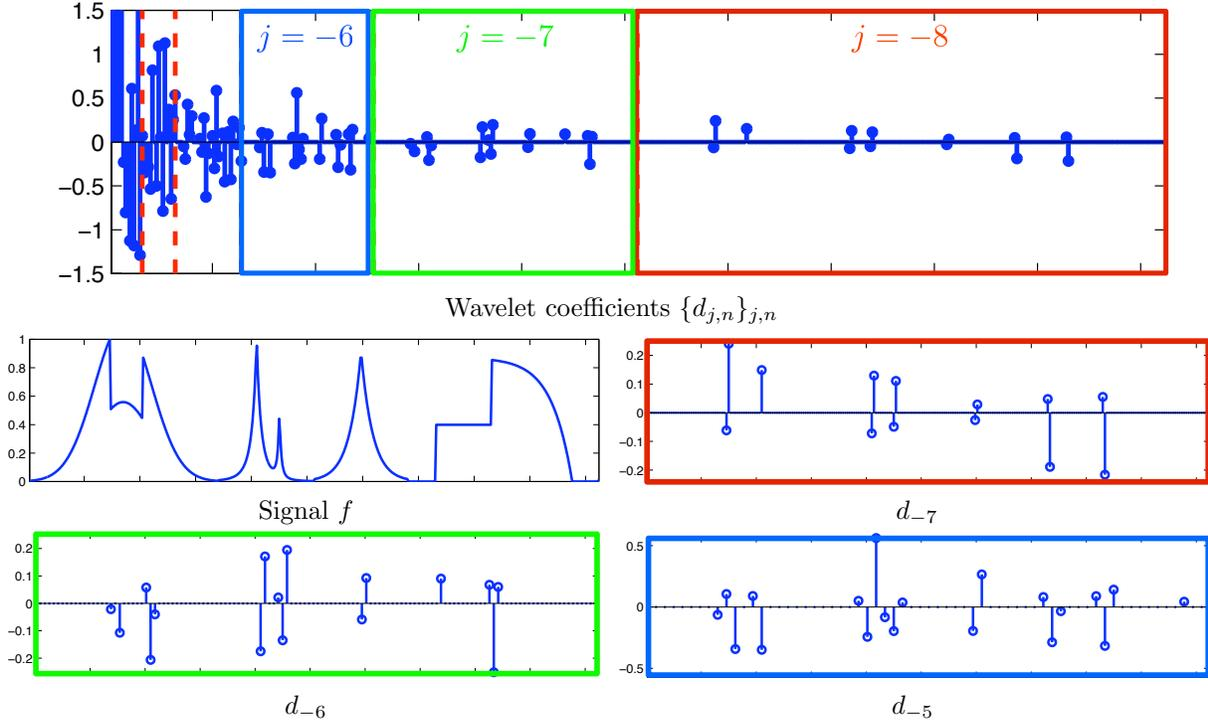
Figure 3.8: Wavelet coefficients. Top row: all the coefficients. Bottom rows: zoom on the different scales
