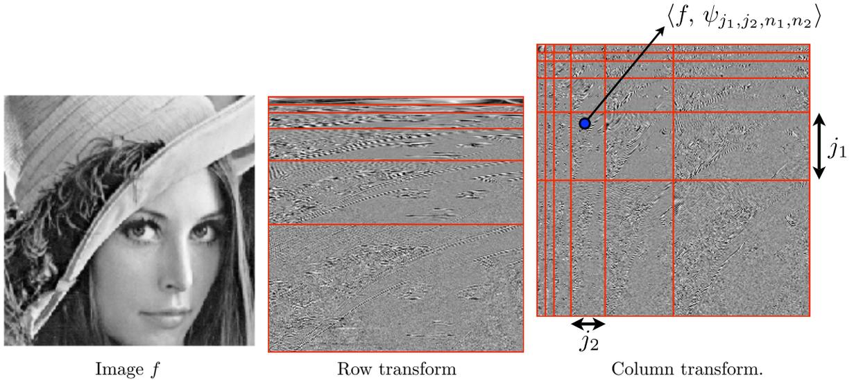
Figure 3.15: Steps of the anisotropic wavelet transform.
