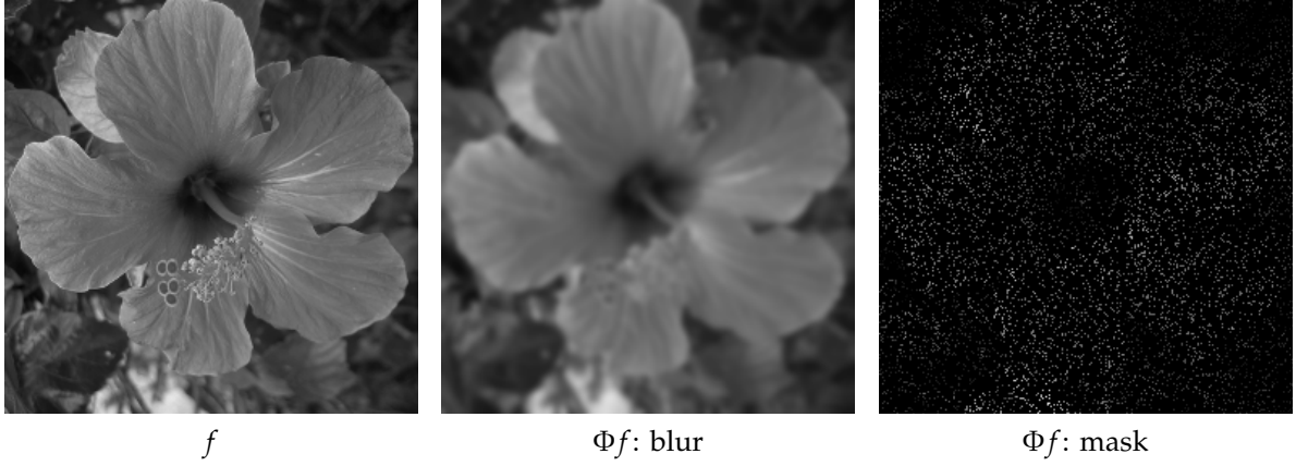
Figure 3.3. Two noiseless observation operators applied to the same flower image: Gaussian blurring and a mask retaining about 10% of the pixels. Missing entries are displayed in black.
